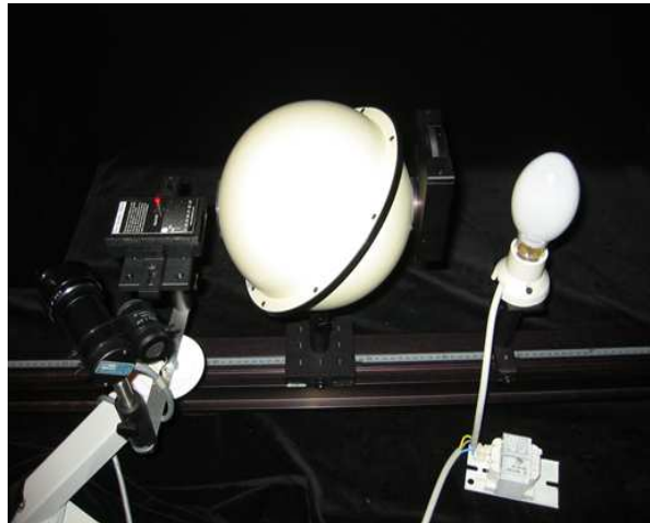
Fig. 19.— The Variable Low Light Level Calibration Standard. From left to right are visible the SQM and the reference detector, the Uniform Integrating Sphere, the aperture wheel and a test lamp for road lighting (baffles removed). Spectral irradiance/radiance standard lamps with radiometric power supplies and optical devices are used in other configurations.
